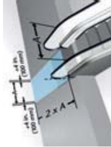
Figure 6.1 Passenger circulation area for single escalators A = distance between handrail centerlines
